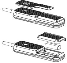
2. Replace the battery cover and screw the cover into place. Finally, screw the belt clip on.
